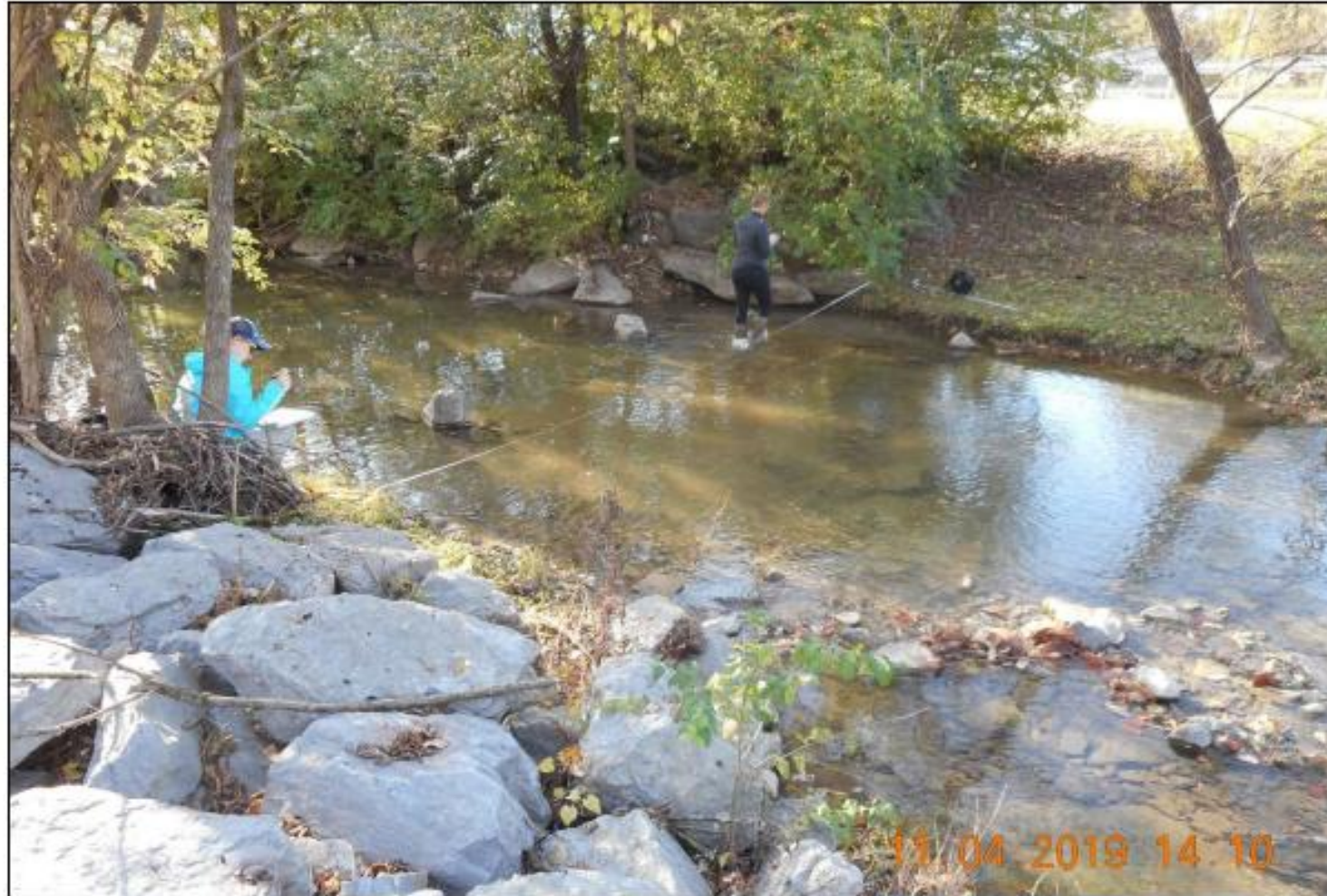
12 of 14: CHL conducting stream gauging upstream of seep #1
