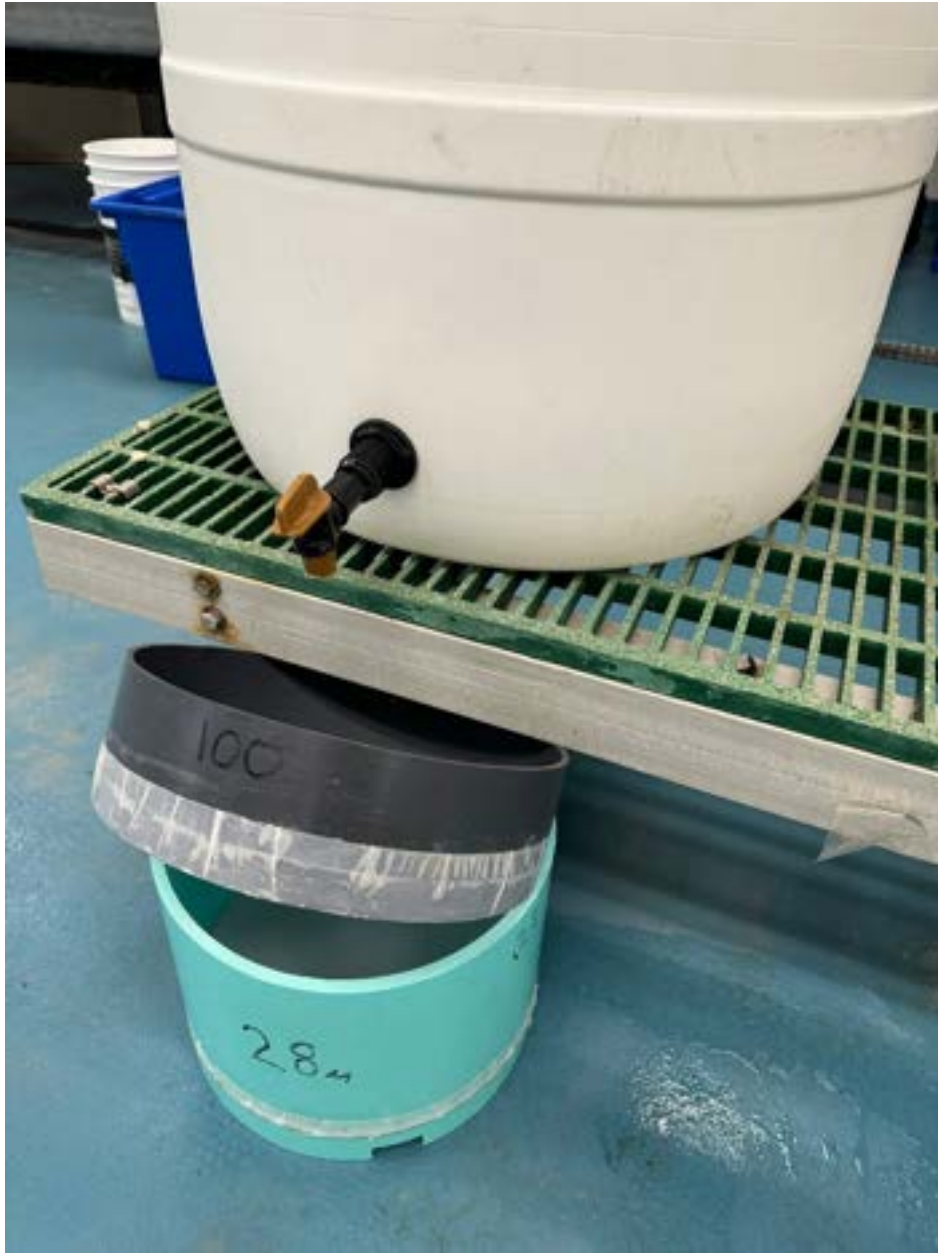
Figure 6D. Bin-silo drain-down setup. After running a trial, each replicate barrel was drained down onto a 100 \mu m and 28 \mu m mesh sieve. All contents sitting on the 28 \mu m sieve were promptly rinsed into a clean bucket and examined under a microscope for potential larval collection.
