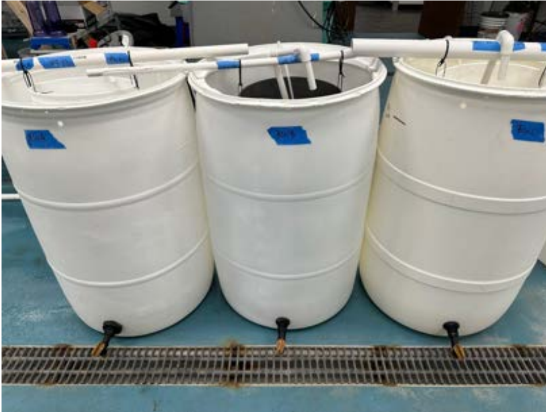
Figure 6A. Bin-silo barrel setup. Each trial consisted of three replicate barrels that contained a downweller airline to recirculate water and introduce air into the barrel for the duration of the trial. At the end of each trial, all barrels were drained down on a 100 \mu m and 28 \mu m mesh sieve.
