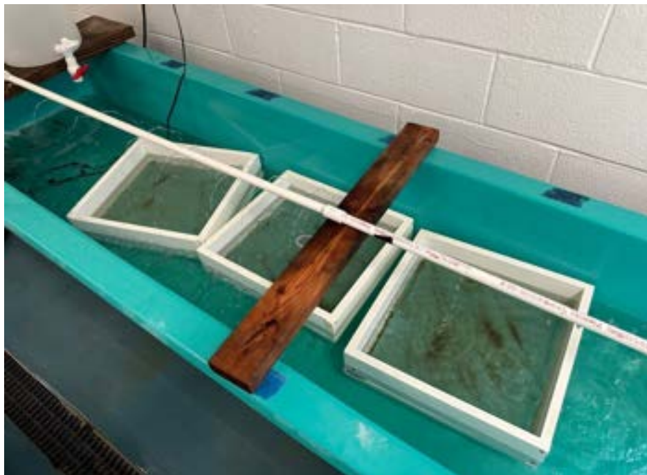
Figure 6F. Ribbed Mussel downweller tank set up for post-set ribbed mussels. A PVC water circulator and airline constantly pumped water on top of the mussels. This design proved ineffective at holding the animals due to their ability to crawl over the side walls.
