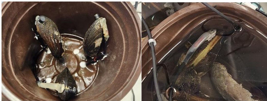
Images 1-2. From left to right. Image 1 displays a group of 3 ribbed mussels freshly attached to hall effect sensors and magnets. Mussels are held in an upright position in a planter through the attached hall effect sensor having been zip tied to a slit in the planter. Mussels are placed in such a way that the magnets do not interfere with each other. Image 2 displays an apparently acclimated mussel with extended byssal threads and a partially open valve.
