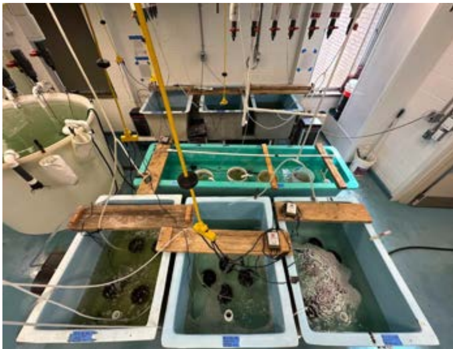
Figure 3. Broodstock conditioning tanks at the Flax Pond hatchery. Ribbed mussels were housed in planter pots held at 20°C and continuously fed a mixed microalgae diet. Air stones and pumps were used to circulate water.
