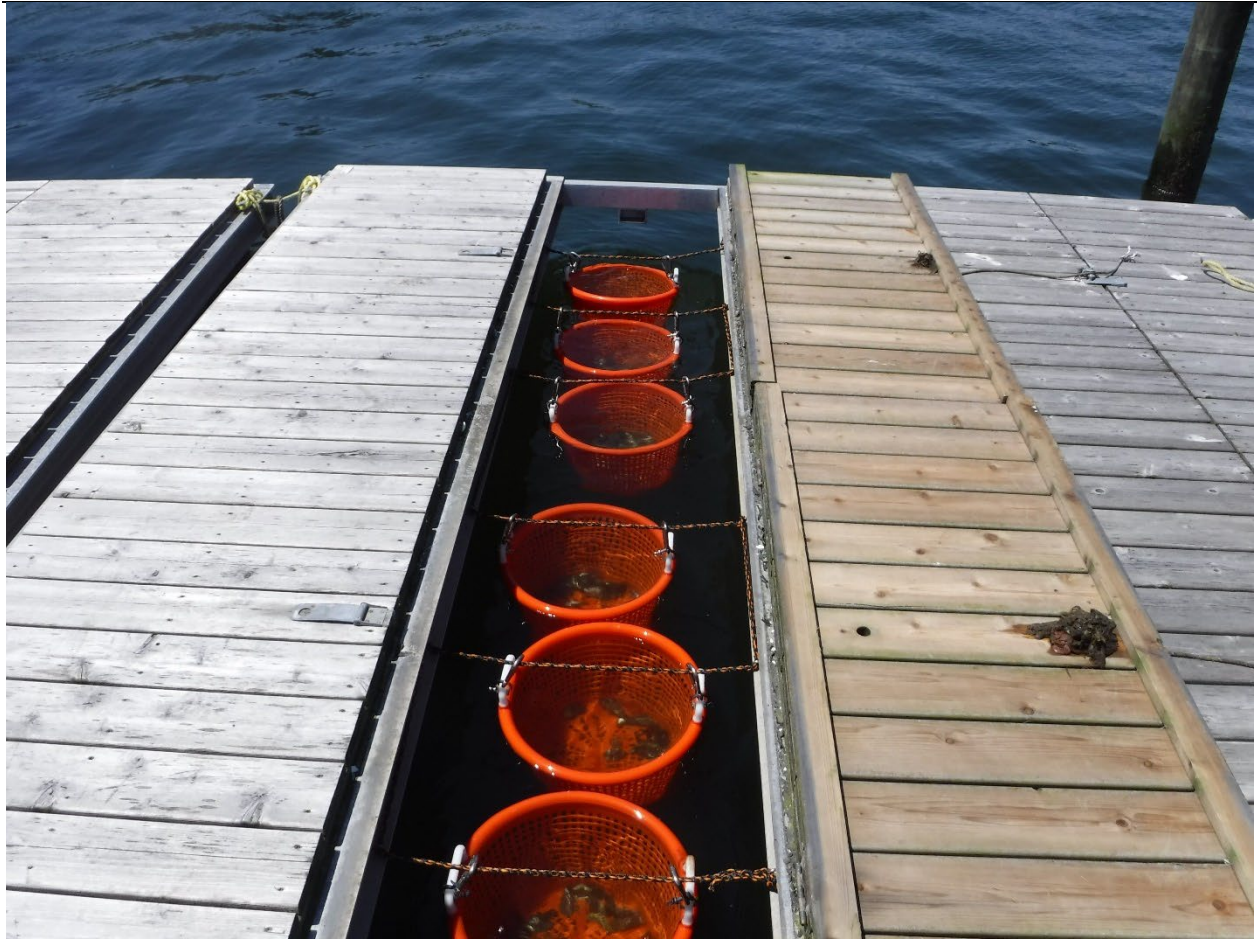
Figure 17. Field grow-out set-up. Floating docks were installed at both the Huntington Harbor and Northport Harbor sites in early April for use during Year 1 of the study and removed at the end of the season in November. On the dock, the wild-collected adult ribbed mussels were placed in orange fish baskets and hung beneath locked trap doors at the start of the study, monitored twice a month and cleaned as needed, but otherwise left undisturbed for the project period. This set up was repeated in Year 2 with hatchery-cultured juvenile mussels. Photo courtesy of Barry Udelson, formerly at Cornell Cooperative Extension and currently at NY Sea Grant.
