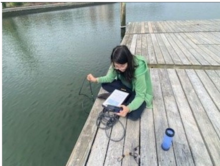
Figure 19. Water quality measurements, such as temperature, salinity, and pH, were taken at each site using a multiparameter sonde. Photo courtesy of Johanna Mazer, former Nutrient Bioextraction Coordinator Assistant.
