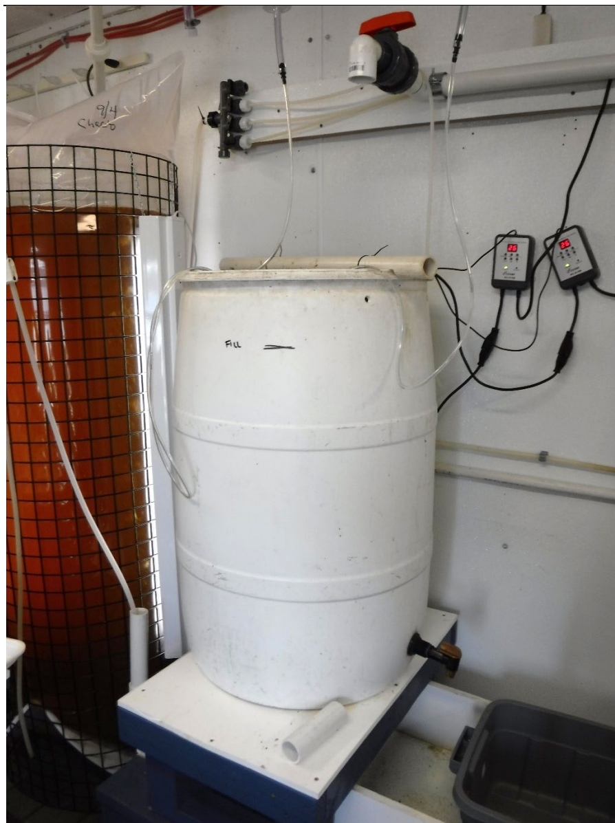
Figure 10. The bin containing the mesh-bottom silo and adult wild-collected ribbed mussels. This set up was used for spawning gametes using the Bin-Silo method developed at Rutgers University. Photo courtesy of Barry Udelson, formerly at Cornell Cooperative Extension and currently at NY Sea Grant.
