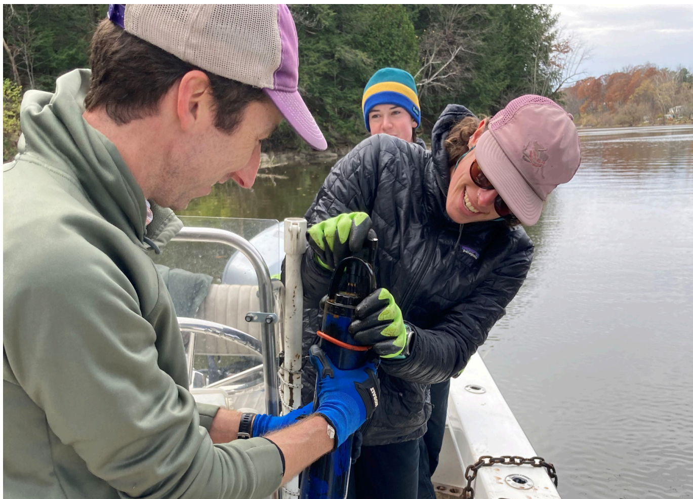
Matthew Vaughan and Kelsey Colbert using a multiparameter sonde at the long-term monitoring buoy in the Lamoille River, Vermont. Photo credit: Lake Champlain Basin Program.
