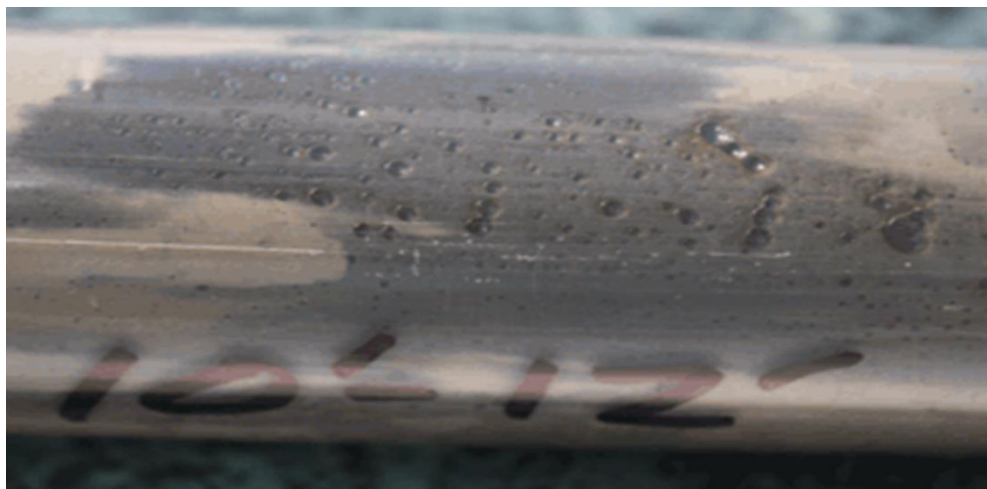
Figure 1. Picture of a soil core taken from a petroleum contaminated site, showing microbially-driven geochemical changes, including precipitation of black metal sulfides and biogas formation (CO 2 and methane bubbles). These biodegradation processes, collectively known as natural source zone depletion, are common at most petroleum contaminated sites. Quantifying the rate of these processes is key to the LNAPL conceptual site model. Measured NSZD rates can vary by as much as 10x, depending on the methodology used.
