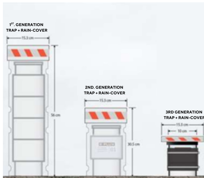
Figure 2. From left to right, first, second and third generation CO 2 trap and rain cover designs. Small deviations from the stated dimensions may have occurred in a few cases, as changes from first generation to second were iterative.
