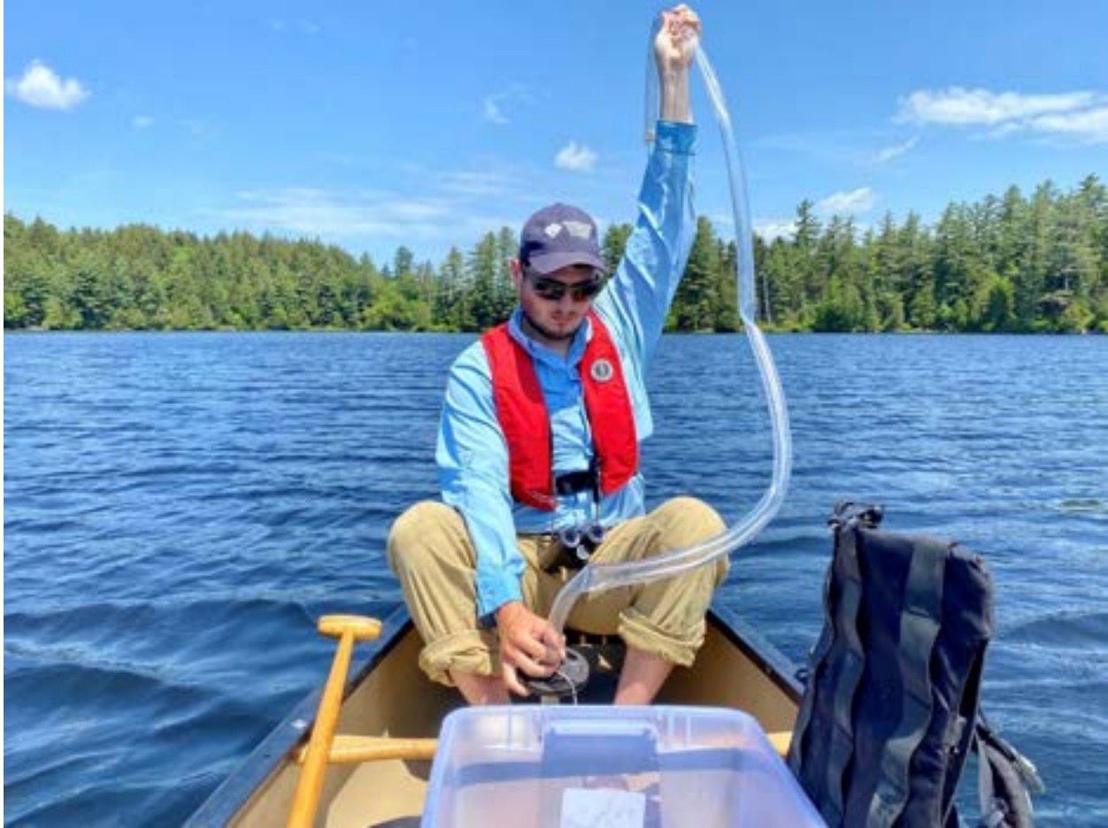
Photo 4. Paul Smith's College Adirondack Watershed Institute Research Technician, Connor Vara, collecting an integrated tube sample.
