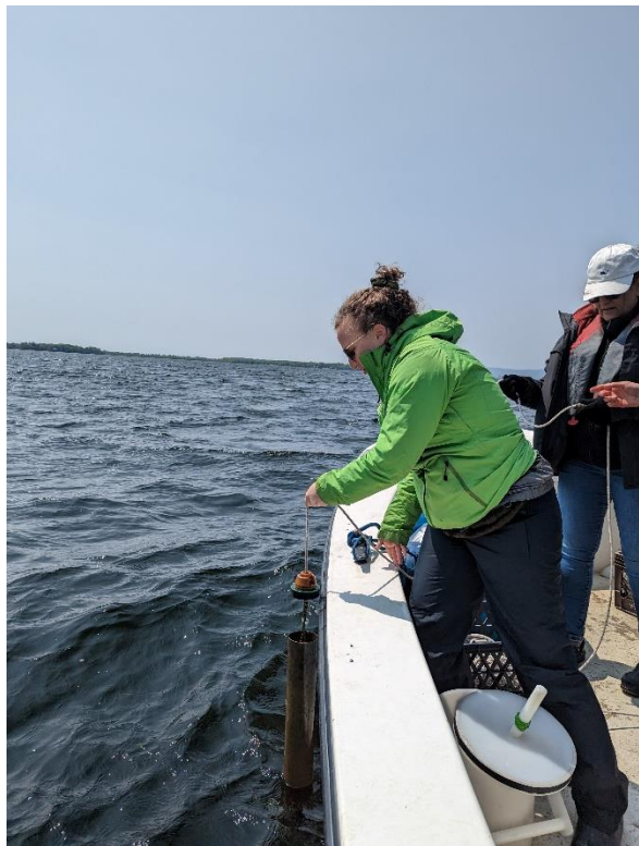
Emily Bialowas collects water quality samples with a Kemmerer sampler.
