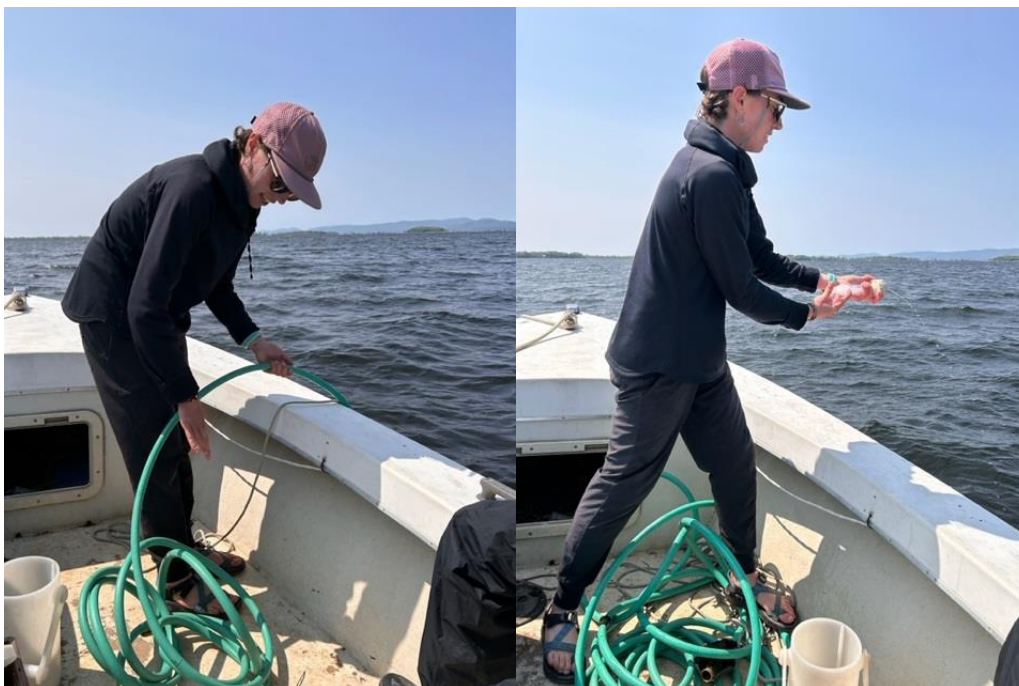
Kelsey Colbert collects an integrated sample of water down to 2x the Secchi depth, and sends it through a filter for chlorophyll-a sample collection.
