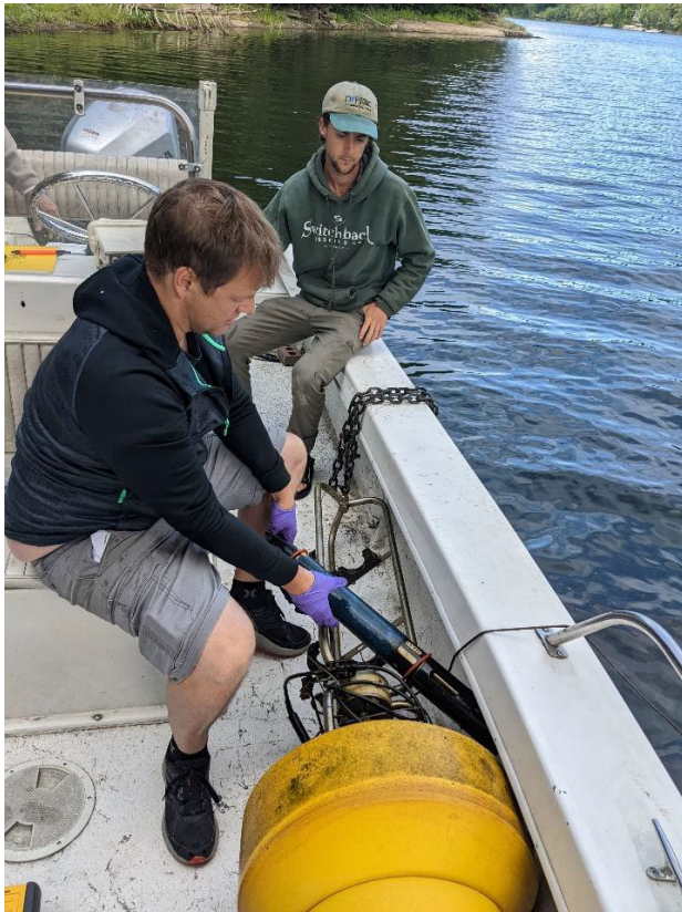
Peter Isles (front) and Connor Quinn (back) remove the multi-parameter water quality sonde from the buoy housing for cleaning and sensor calibration.
