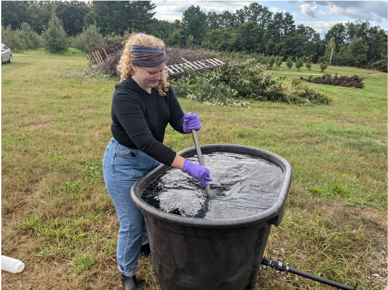
Sam Brewer combines the concentrated pollutant mixture with “clean” groundwater to create the synthetic stormwater.
