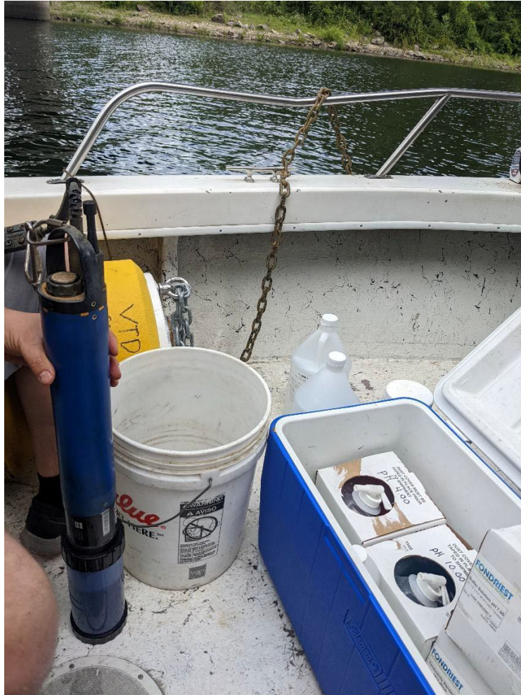
YSI EXO2 multi-parameter water quality sonde and calibration standards.
