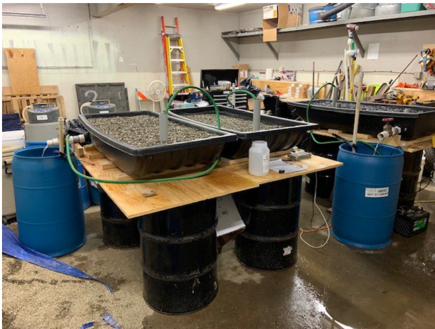
Figure 10. Three filter sleds recirculating P solution
