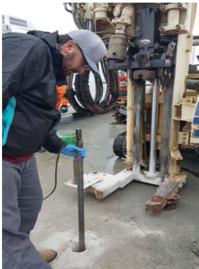
A Columbia Technology field tech inserting the membrane interface probe into a bore hole.
