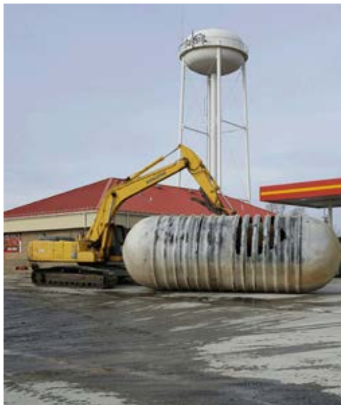
Excavated, exposed, extracted and accompanied by the backhoe that lifted it from the pit, the failed tank sits only a few feet to the east of the hole from which it emerged. The delaminated ribs are fairly obvious on the right side of the tank.
