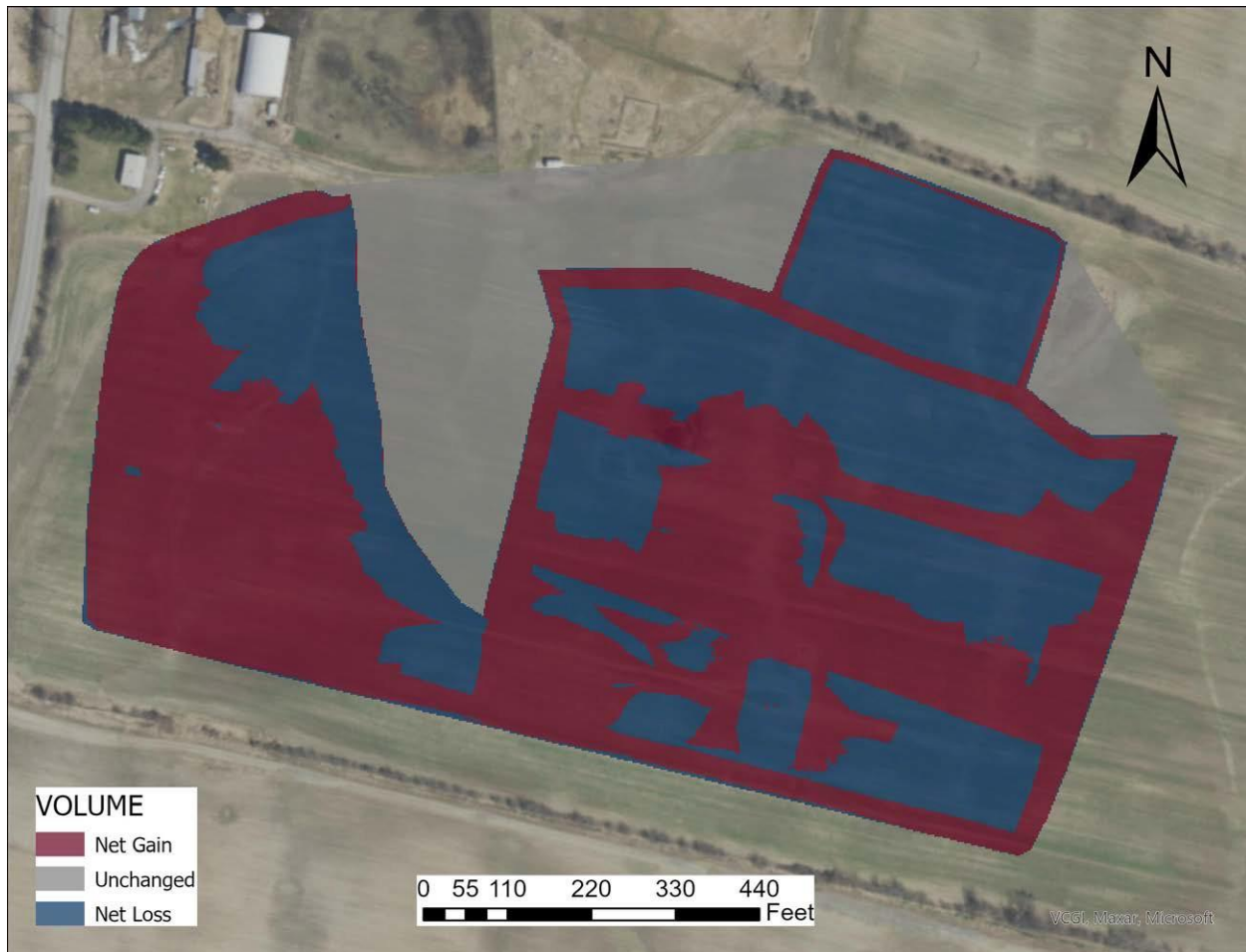
Figure 30. Cut and fill diagram for the Dunsmore 1 site facility
