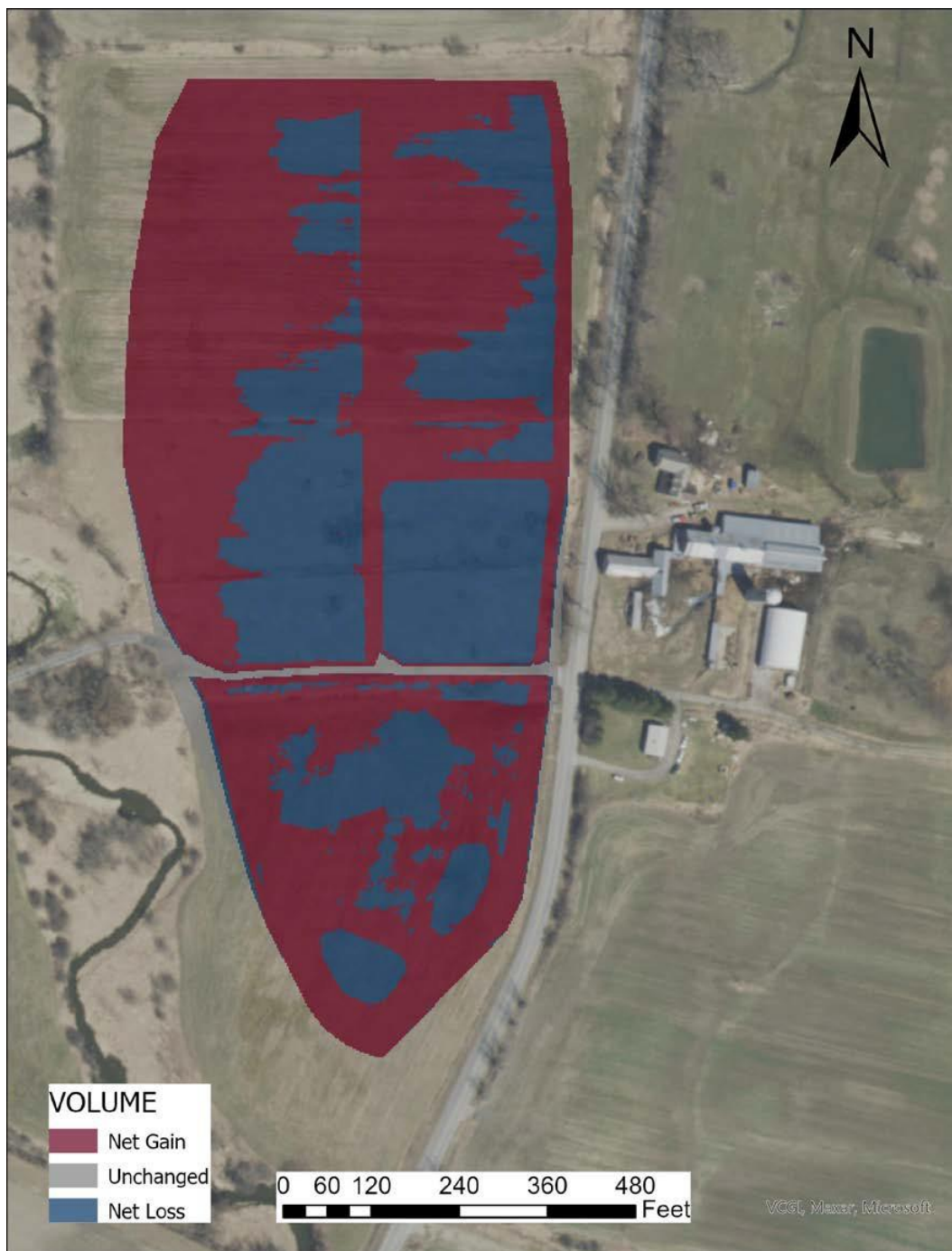
Figure 33. Cut and fill diagram for the Dunsmore 2 site facility
