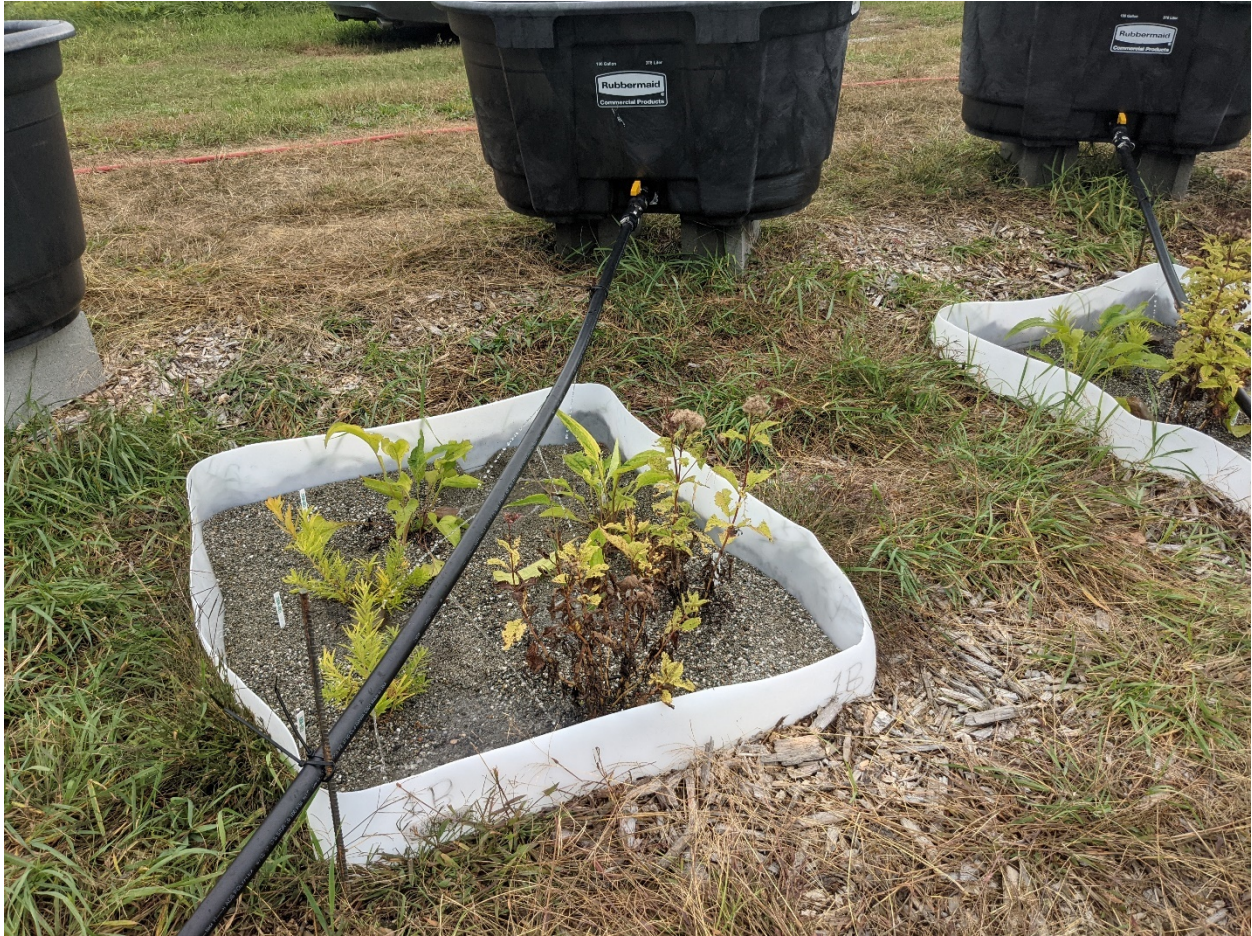
A close-up view of an experimental bioretention basin during a simulated rainfall event.
