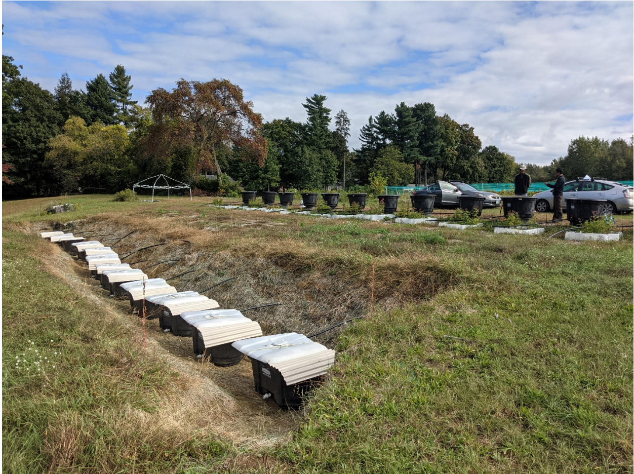
A full view of the experimental site. The lower storage containers catch simulated rainfall event effluent for sampling.
