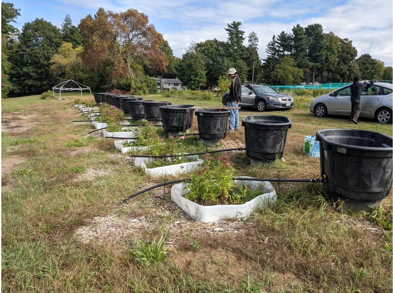
Synthetic stormwater tanks rest above experimental bioretention plots before the simulated rainfall event.
