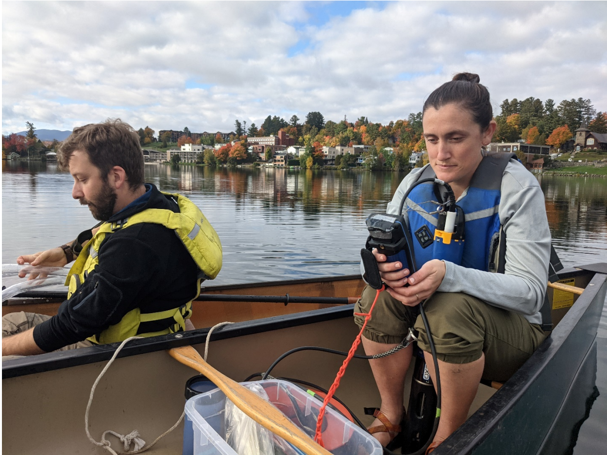
Brendan Wiltse collects a 2-meter integrated water sample, and Sue O'Reilly prepares to make water profile measurements of dissolved oxygen, specific conductance, and pH at 1-meter intervals using a hand-held water quality sonde.
