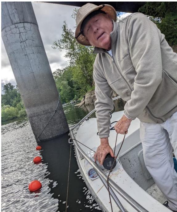
Pete Stangel uses a winch to raise the buoy anchor for maintenance.
