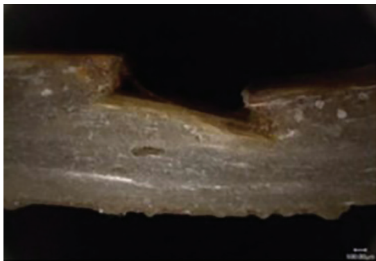
Figure 7 Magnified groove cross section showing sand particles and a void space.
