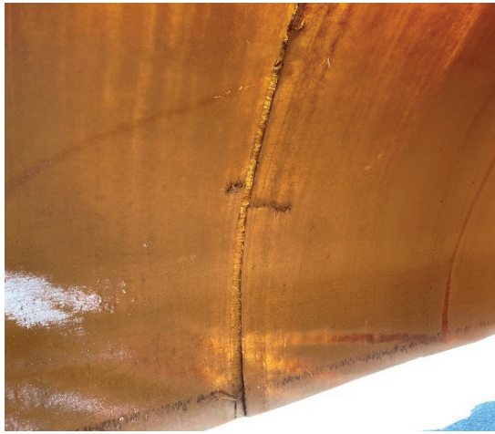
Figure 5 View of inside of the FRP UST sample that was collected showing the groove.
