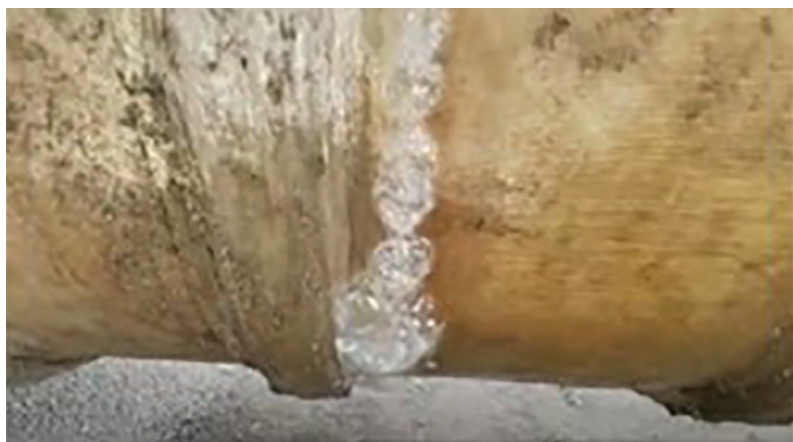
Figure 3 Bottom of the FRP UST during the pressurized soap test showing the location of the crack.
