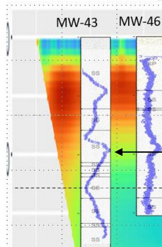
Subtle EC increases detected with borehole logging not seen in surface ERT
