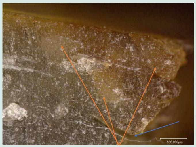
Orange arrows show where gasoline has permeated the gel layer changing the color. Notice color near the crack vs to the left. Blue arrow is another crack perpendicular.
