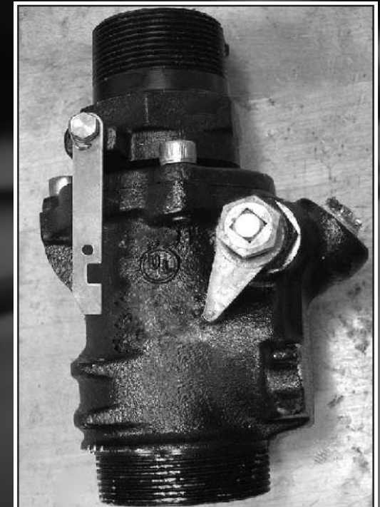
FIGURE 10-1. When activated by fire or impact, the shear valve closes and blocks fuel flow from the dispenser supply lines. The shear valve shown is in the closed position.
