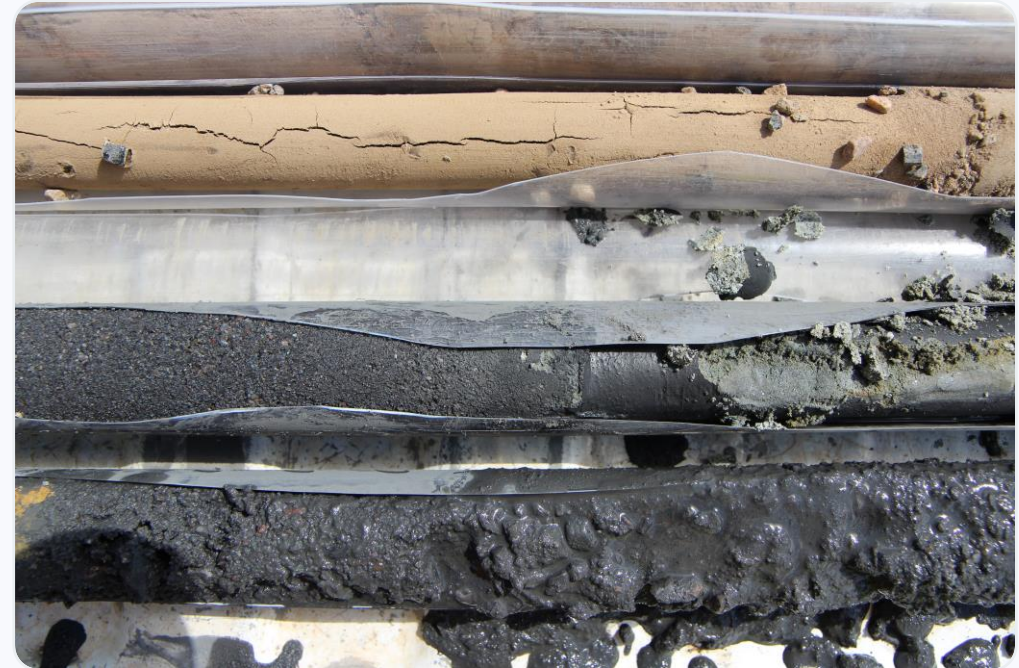
Soil core collected across the injection interval (bottom 2 core samples) showing successful distribution in sandier flux zones.
