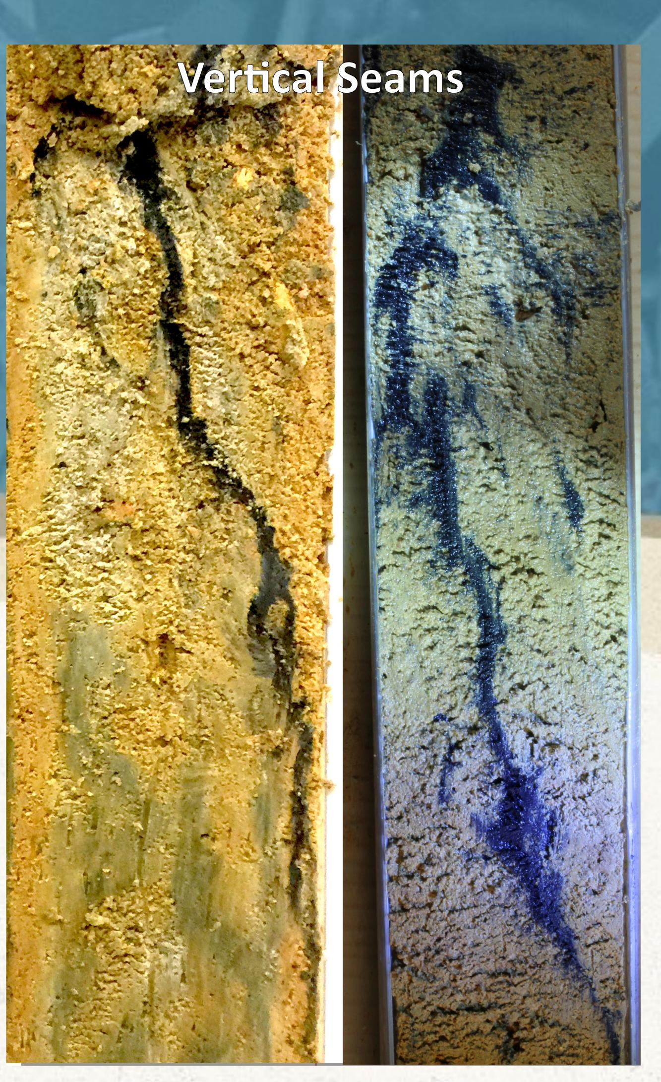
Site geology precluded traditional DPT from being utilized for injection, due to dense silty sands, gravels, and glacial till at depth. An innovative proprietary drilling and injection process (GeoTAP™) was used to access targeted depths This process also provided a complete soil profile, which allowed the determination of succinct top and bottom injection spans for each injection point within the transect.
