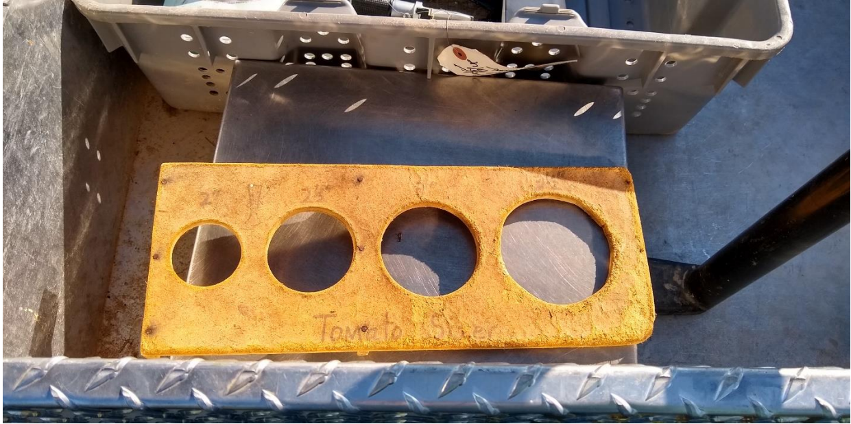
Tomato sizing device used to sort tomatoes.
