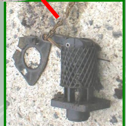
Leaking Drain Valve
