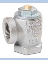
**Mechanical Anti-Siphon Valves (ASV)** are designed to withstand a specified negative head pressure to prevent the contents of the tank from being siphoned out in the event of a line break below the fluid level. As with the solenoid valve above, the ASV should be placed at the high point of the fuel line.
