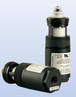
**Mechanical Line Leak Detectors (MLLD's)** test the underground portion of piping from the UST to the solenoid valve in the Onshore Transition Sump at the beginning of a fueling process. MLLD's detect a leak rate greater than 3 GPH @ 10 PSI.
