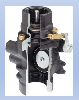
**Emergency Shear Valves, or Impact Valves** are installed beneath the dispenser in the sump. These valves protect against a fuel release if the dispenser is impacted. The shear section will break, causing the spring-loaded hold-open arm to slam closed. The hold-open arm is held by a fusible link which will melt at 165 degrees F.
