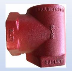
Leak Detector Tee may be used to install the MLLD or ELLD downstream of the anti-siphon valve in the UST sump. Leak detector tee's have special threads to accept the leak detector in the designated port, with a direction specific inlet and outlet port.
