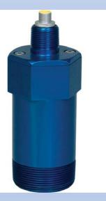
**Electronic Line Leak Detectors (ELLD's)** test the underground portion of piping similar to MLLD's, but at the conclusion of a fueling process rather than the beginning. ELLD systems are capable of detecting 3 GPH catastrophic leaks, as well as performing precision 0.1 / 0.2 GPH line leak testing.
