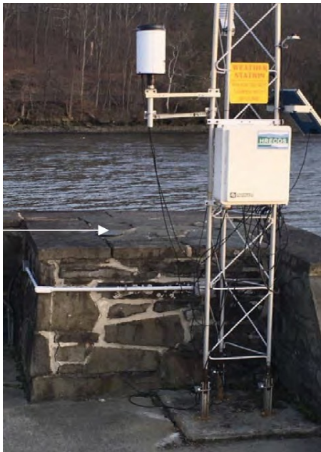
Figure 7.14 Weather station at corner of patio. White instrumentation box was moved up one rung on tower the day before surge. Arrow indicates benchmark and approximate highwater. (Source: DEC, HRNERR)
