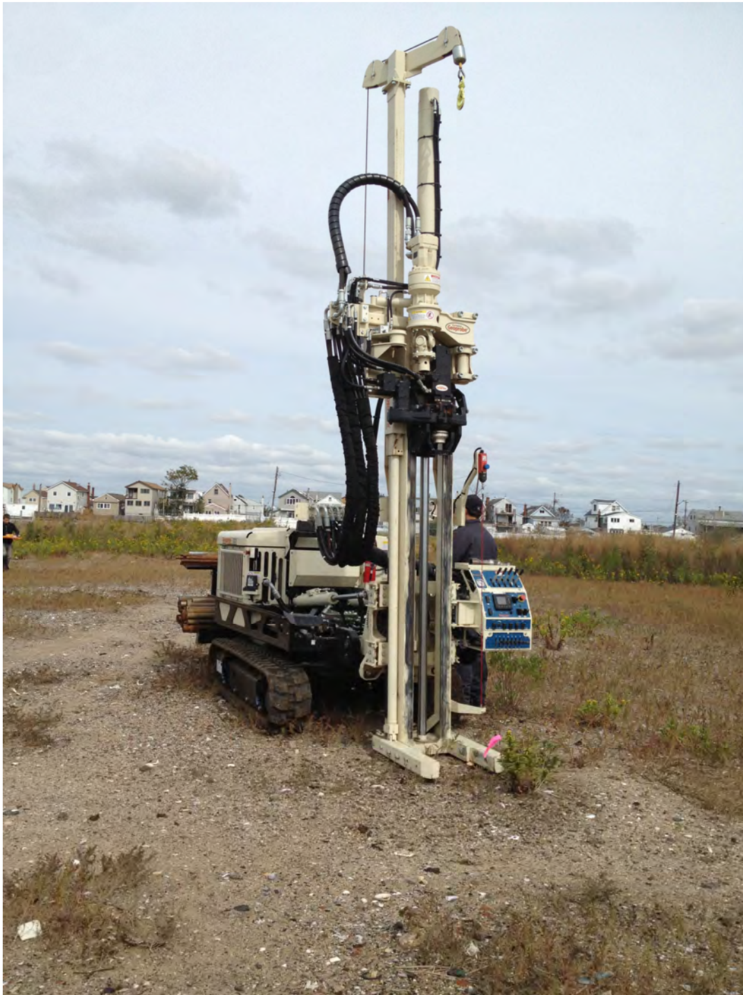
Photo 2 - Sampling using Geoprobe drill rig. View is towards the north.
