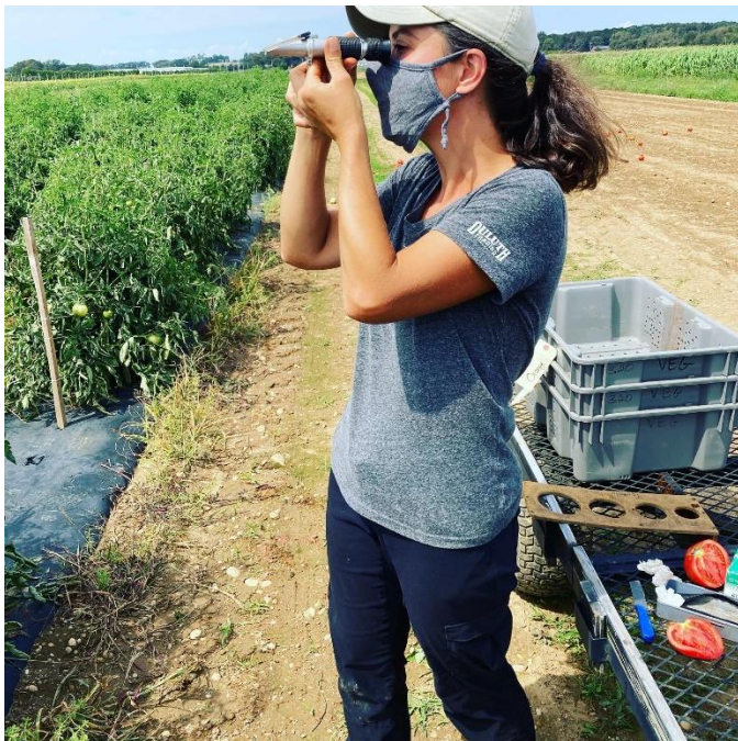
Image 7. A refractometer being us to measure the degrees Brix of a fresh tomato. Degrees Brix measures the sugar content of an aqueous solution.
