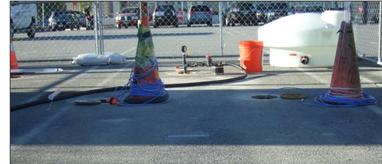
Continuous “down-hole” specific conductivity measurements
