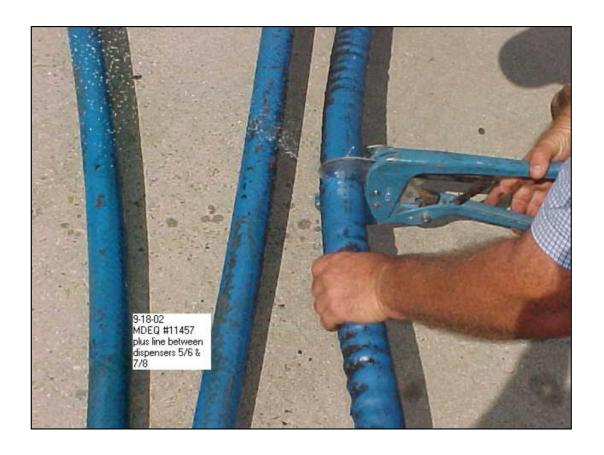
Product leaking through the primary pipe sometimes became trapped between the primary and secondary walls of Omniflex. In this photo, fuel is spraying out of the interstitial space between the walls of the pipe as the pipe is cut.
