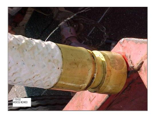
Fuel sometimes became trapped within the layers of Enviroflex pipe. In this photo, fuel is draining out of a pinhole in the outer covering even after the piping itself has been emptied of fuel.
