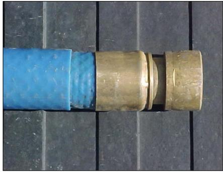
Total Containment Omniflex pipe consisted of either the model 1501 or 1503 primary pipe with a blue outer jacket that provided the secondary containment. Omniflex pipe could be buried directly in the ground or it could be installed within the 4 inch diameter secondary pipe used with Enviroflex.
