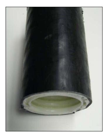
Marinaflex was manufactured by adding carbon black to the outer jacket of Omniflex pipe. The carbon black provided some protection from degradation due to exposure to sunlight.
