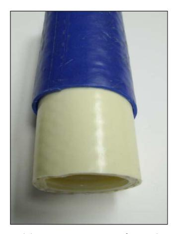
Model 1502 piping was manufactured specifically for Amoco. The primary pipe was thicker and had a smooth outer surface.
