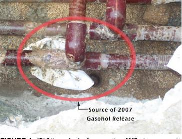
FIGURE 1. "T" fitting under the dispenser where 2007 release occurred.
