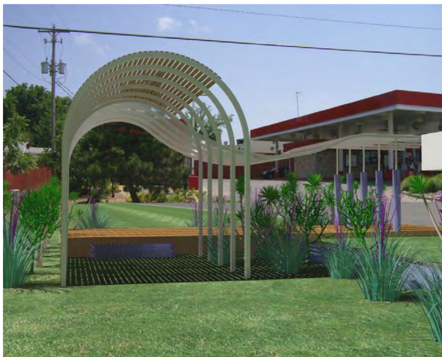
Architectural rendering by Neil Steiner and Peter Zuroweste, University of Kansas, showing the rain garden and sustainable pavilion that will be built behind Zarco 66 Earth Friendly Fuels. The rain garden will reduce stormwater runoff from the site.
