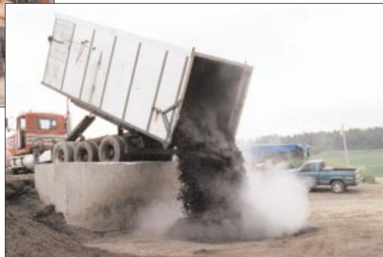
After three days of “cooking,” a mixture of septage, grease, and pine shavings emerges hot, steaming, and sweet-smelling from one of PJI/Tri-City’s composting containers.
