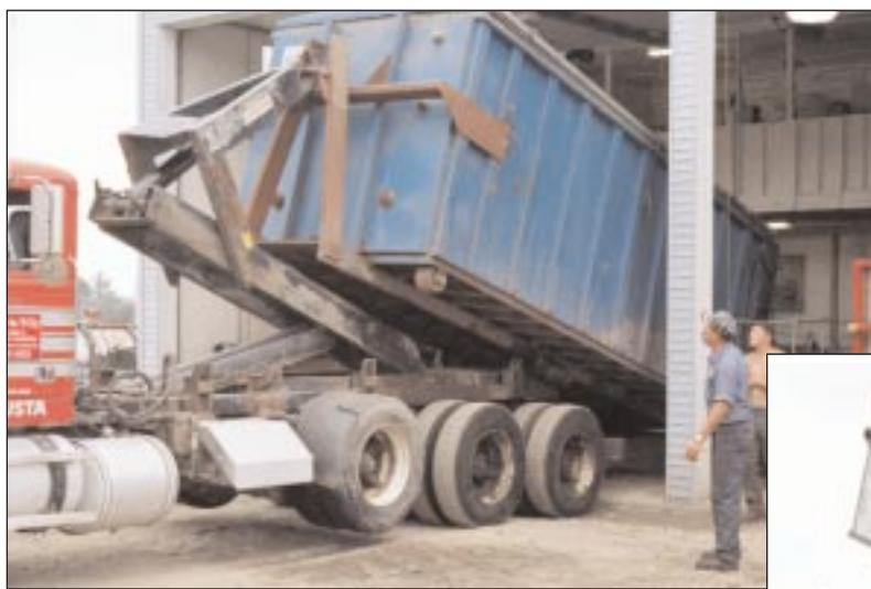
At the Pat Jackson Inc./Tri-City Septic Tank Service facility in Belgrade, Maine, a truck prepares to haul a dewatering container—and the dewatered septage that’s inside—to the company’s composting area.
