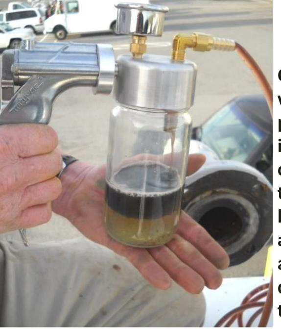
**Checking with a** vacuum sampler can provide far more information on contaminants inside a tank. The vacuum hose can be pulled up after sampling floor and show what is in different strata within tank.
