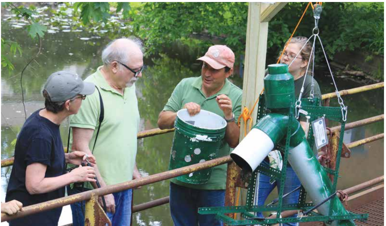
Dan Miller explains the workings of the Sparkill Creek eel ladder in the Piermont Marsh. Miller designed and constructed the ladder, dubbed the "elevator," using materials from a local hardware store. Volunteers use the bucket shown to lift eels over a dam at that site. Also in the photo at right: Sarah Mount.
