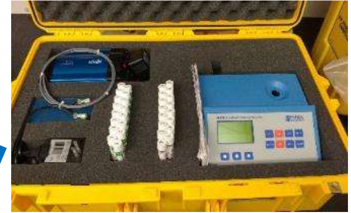
Field analysis (pH, DO, temperature, \text{NH}_4^+ , and \text{NO}_3^- )
