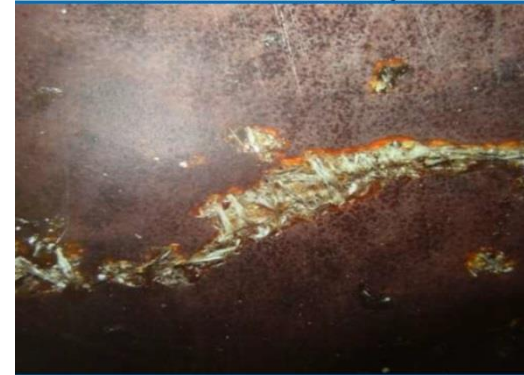
UST 92 Octane interior view: horizontal cracking in tank shell
