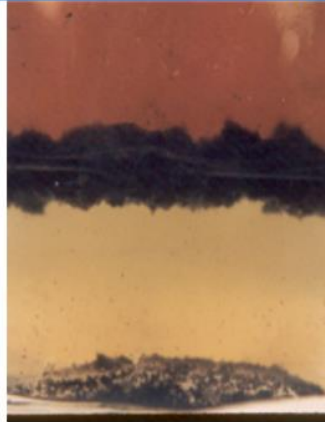
F2. - Diesel Tank Bottom Sample w Microbes
