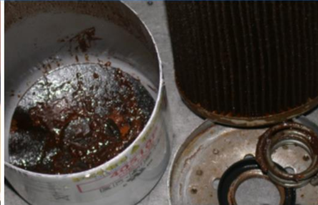
F3. - Corroded Dispenser Filter
