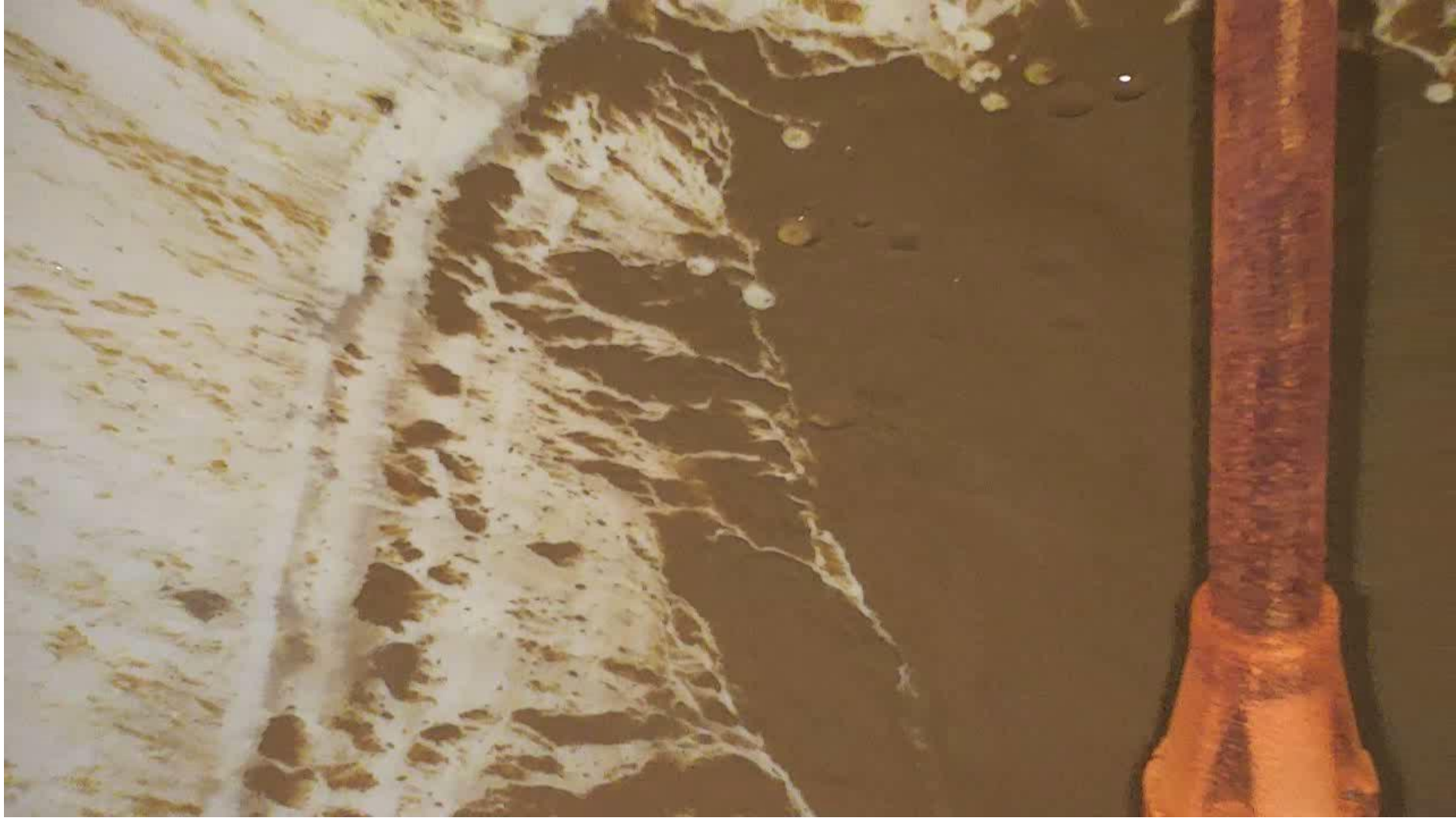
Corrosion on STP Shaft from “Dirty” Ballast Water
