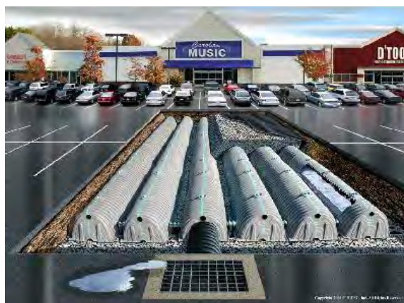
Figure A.11—Rendering of subsurface infiltration structure.
