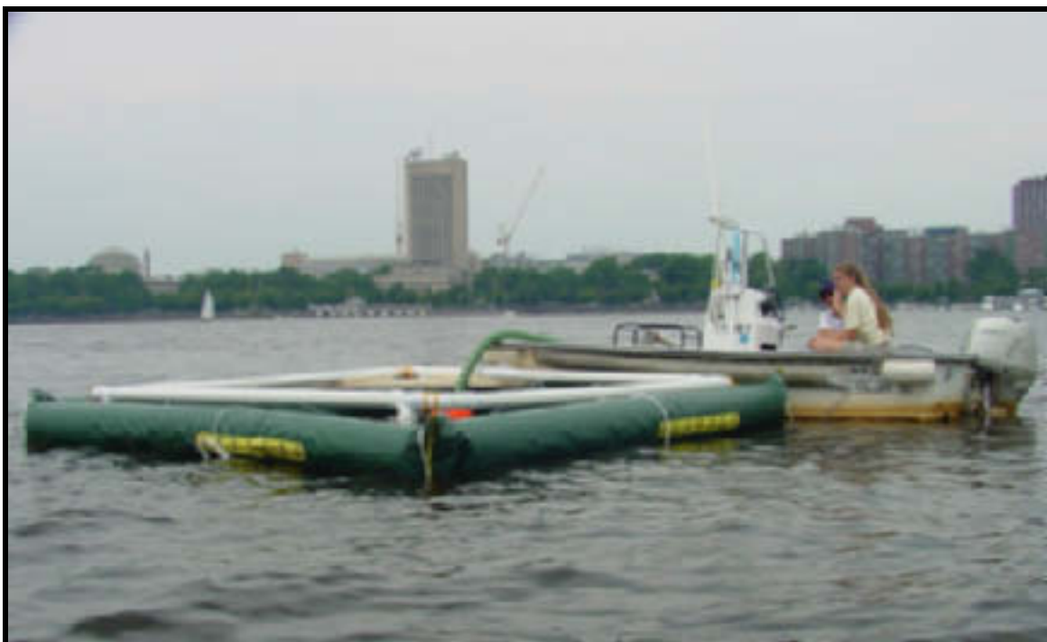
Figure 4. Deployed BPS™ test system with PVC frame submerged.
