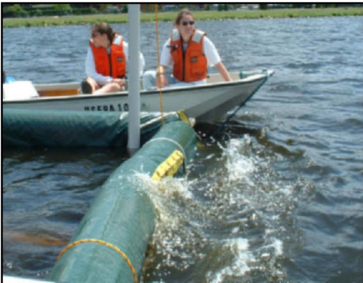
Figure 5. Towing of reefed boom between sites; note splash over on leading edge of boom.
