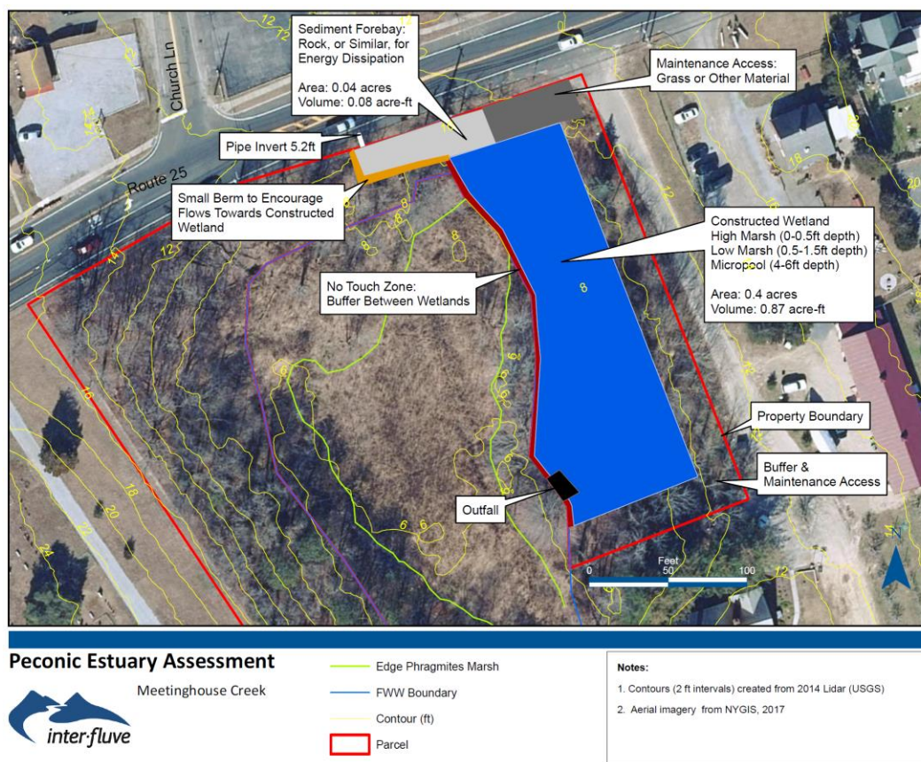
Figure 4: Preliminary Schematic Design for Main Road Stormwater Wetland.
