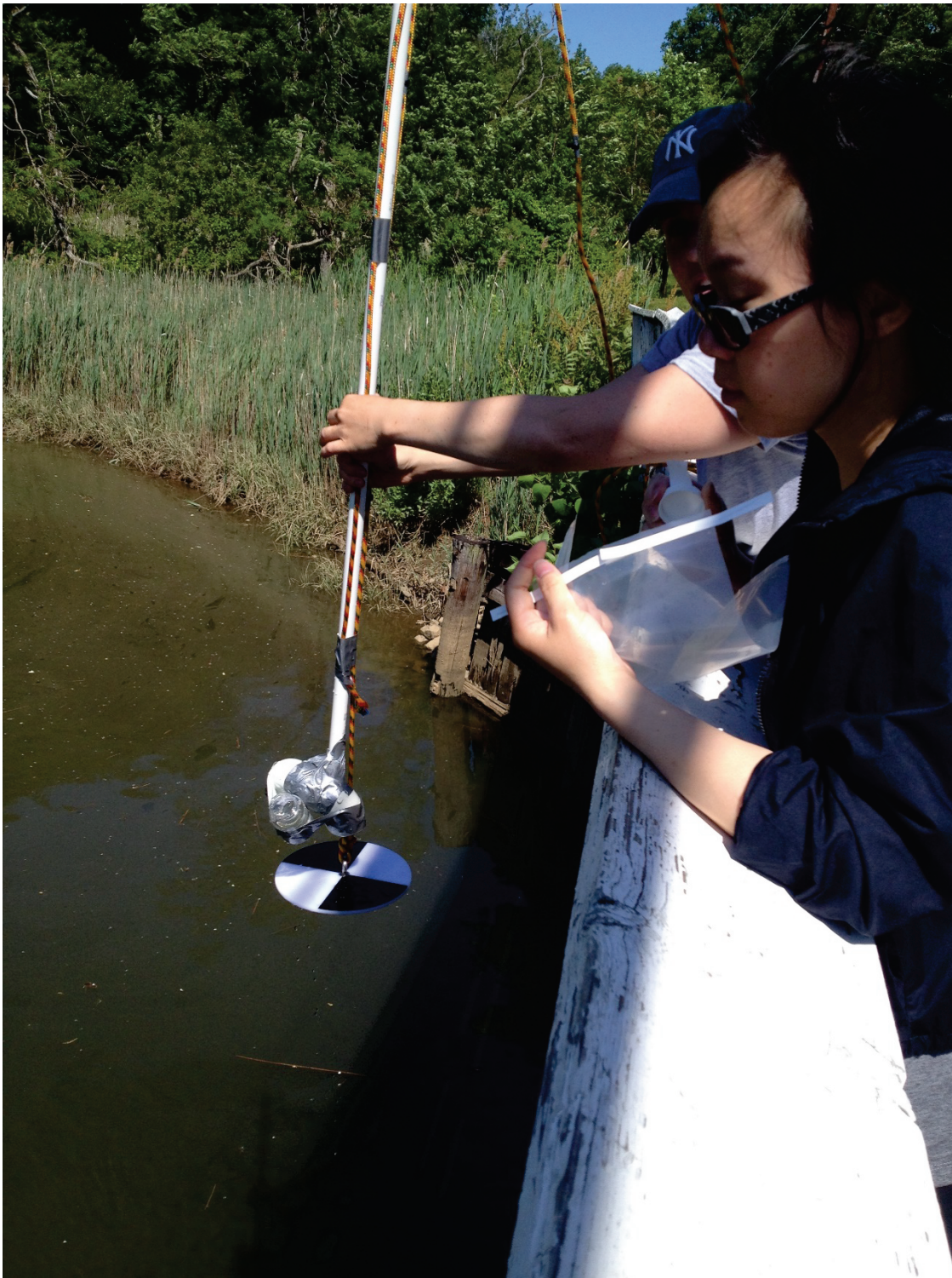
Picture 1 : Summer intern Jia Huang (front) and Dr. A.M. Fitzgerald (back) using a sampling apparatus to gather water sample for Enterococcus testing at site M3 (Matawan Creek), June 2014.
