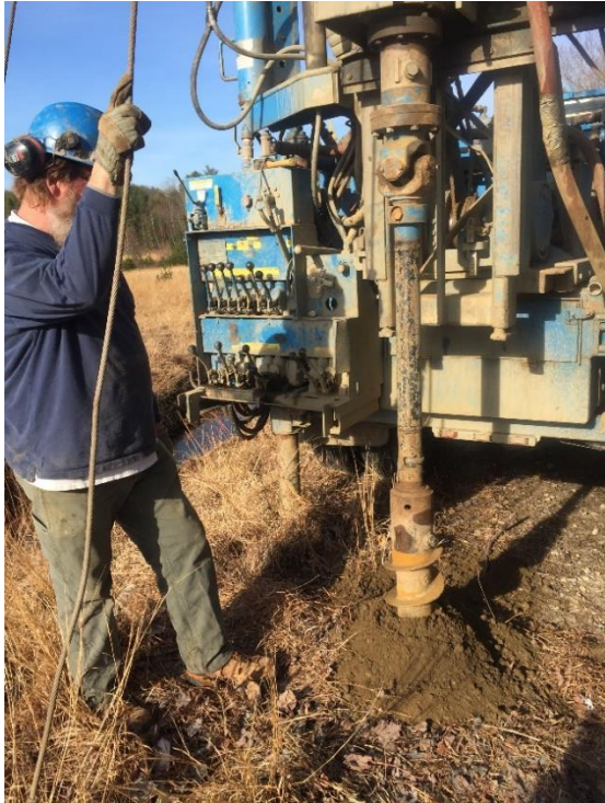
Boring auger digging first soil bore. Soil bores were dug to approximately 20 ft, or if bedrock was hit, which ever came first.
