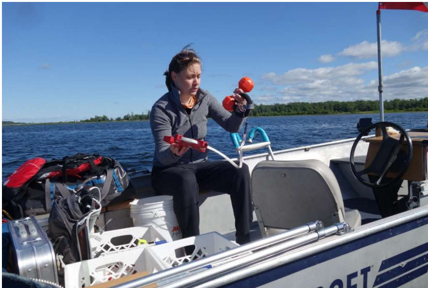
Lauren Sopher, Project Manager, displays the 100ft transect line weighted by a dive ankle weight and one of the surface buoy markers (red hand weight looking object).
