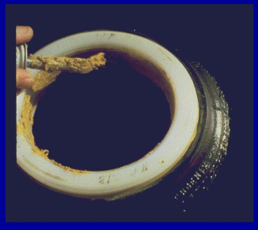
Nylon bushings utilized in all sti-P3 tank bungs to isolate the tank from any other metallic structure.
