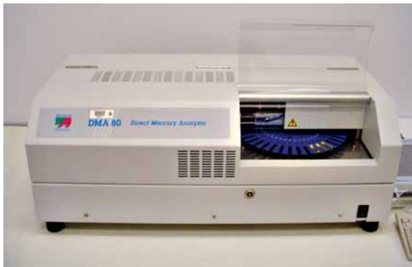
The Milestone mercury analyzer combusts tissue while collecting mercury on a gold column.
