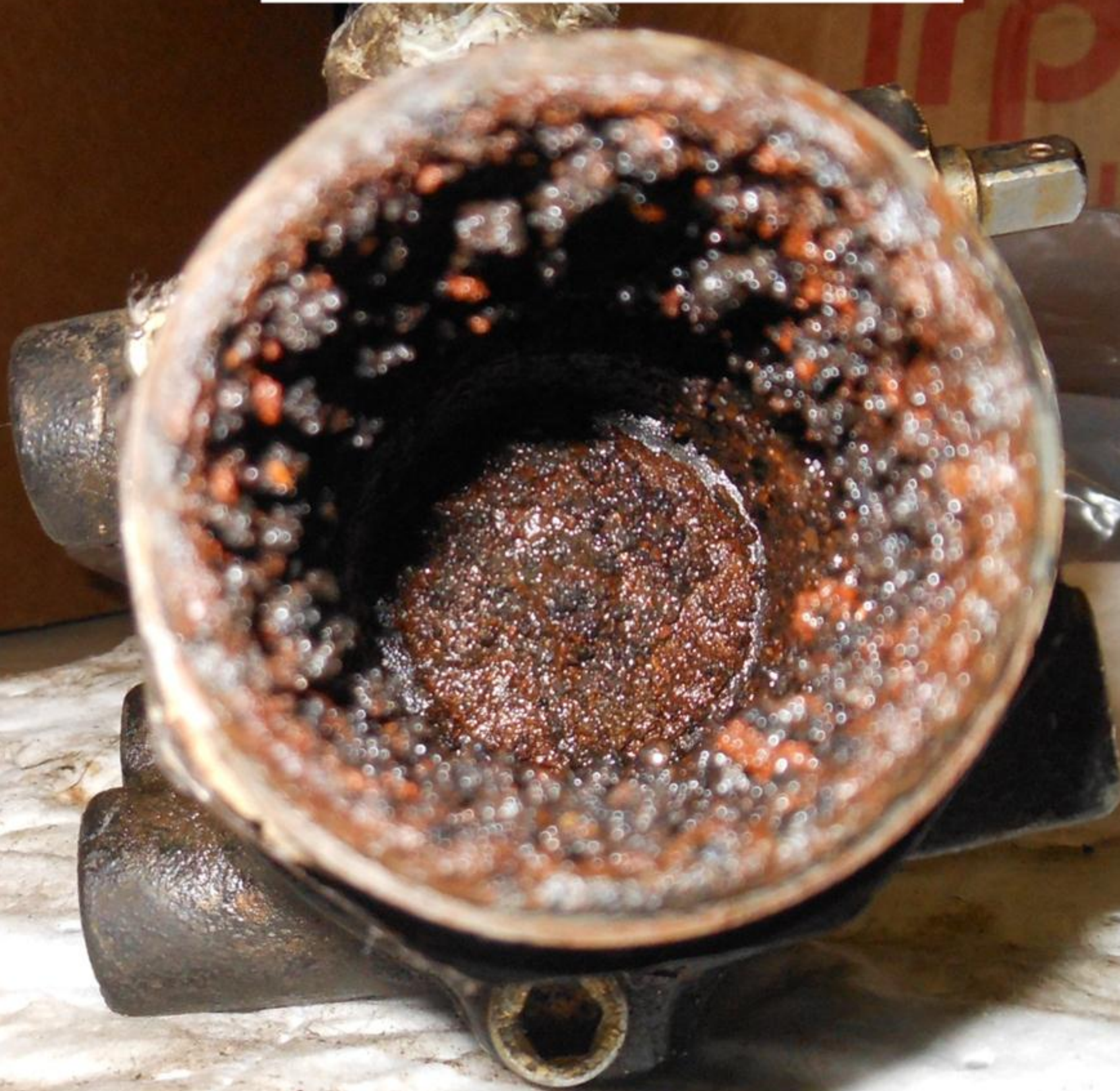
Shear valve internal corrosion
