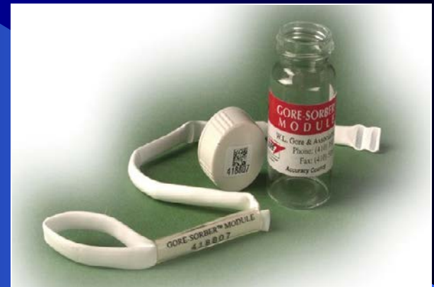
Adsorbent inside vapor permeable, waterproof membrane
