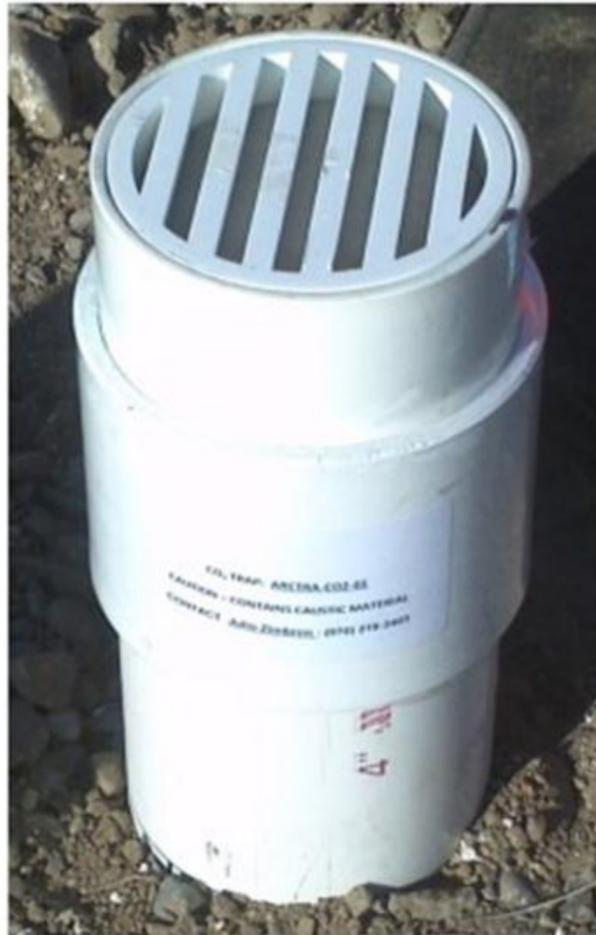
CO<sub>2</sub> sorbent canisters placed on in-ground receiver
