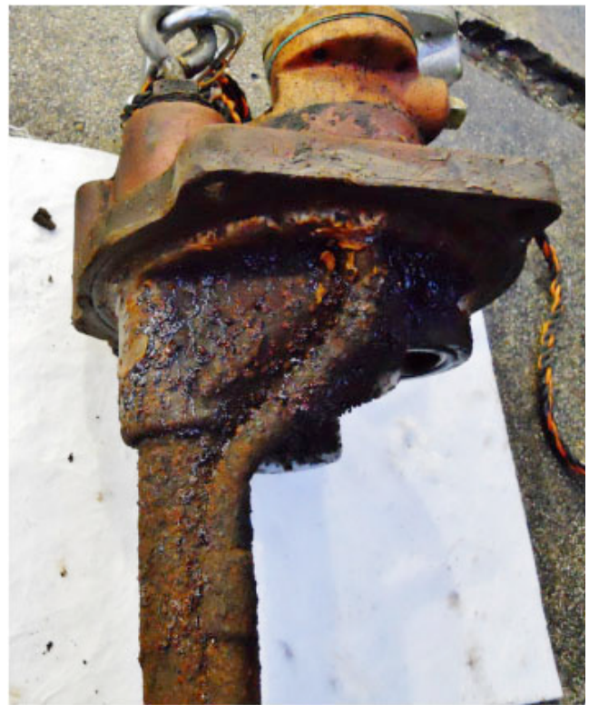
Figure 3. This photo shows the underside of the submersible turbine pump manifold. Although this portion of the manifold is only exposed to fuel vapors, substantial corrosion is present.
