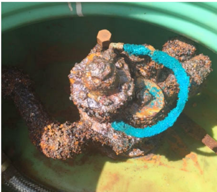
Figure 2. The combination of ethanol, water, and acetobacter produces a very rough looking corrosion product on steel components of tank-top sumps, and a turquoise colored corrosion product on copper components.
