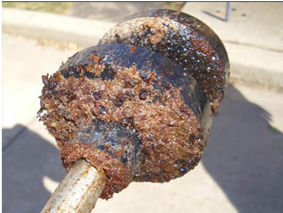
With this kind of crud becoming more and more common in our tanks, it is easy to understand why automatic tank gauging systems need to be looked at periodically.
