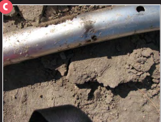
C Area of arcing on the diesel ATG probe tube (by the small hole in the center of the picture).
