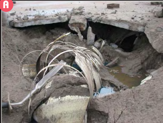
A close up view of the diesel tank. On the right side just under the concrete is the hole in the super unleaded gasoline tank caused by the explosion of the diesel tank. The water level is about four feet below the top of the concrete.
