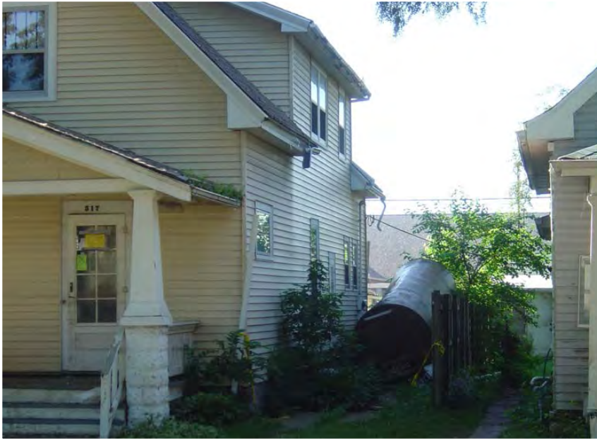
◀ Clark station tank that made it to this neighbor's yard. The tanks were not anchored and empty.
