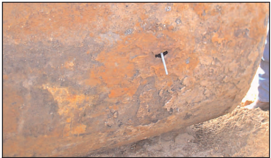
FIGURE 3. The noninvasive assessment methodology did not address the need to provide striker plates in USTs to prevent holes being formed under the drop tubes. For this heavily pitted tank, the noninvasive assessment predicted uniform corrosion.
