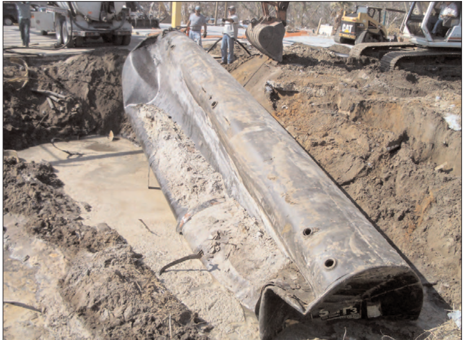
The regular tank buckled and its end caps ruptured.
