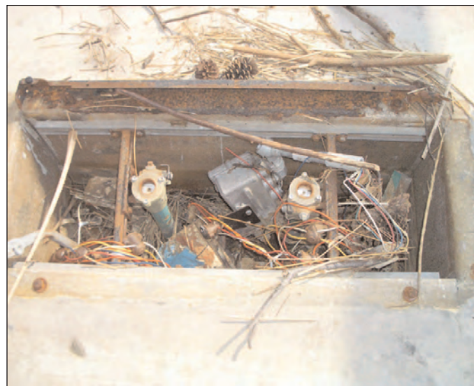
FIGURE 2. This pair of shear valves functioned as designed. The valve mechanisms closed completely and the bottom part of the valves remains solidly anchored to the dispenser island. The top part of the valves, along with the entire dispenser, has been blown away.
