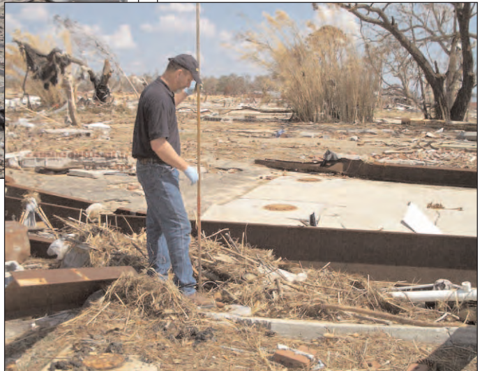
This fill port of a "regular unleaded" tank was uncovered, and the tank was found to be full of water when gauged by MDEQ personnel.
