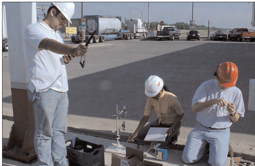
Developing a Low-Cost, Low-Tech Hydrocarbon Sampling Tool. Members of the Southern Methodist University (SMU) Department of Environmental and Civil Engineering conduct a field test to verify the use of a field-detecting device for hydrocarbons in soil. U.S. EPA Region 6 gave the Inter-Tribal Environmental Council a grant to develop a tool that would be portable, low cost, low tech, but accurate (>50 ppm) in detecting the mass of hydrocarbons in soil samples collected and analyzed in the field. The cooperation of the Choctaw Nation helped SMU validate its laboratory-developed data on the tool.
