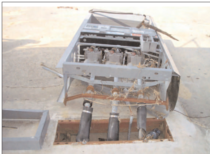
FIGURE 1. This trio of shear valves did not function as designed. The valve body did not separate at the shear joint because the valves, along with their anchoring bar, were pulled up and out of the dispenser island.
