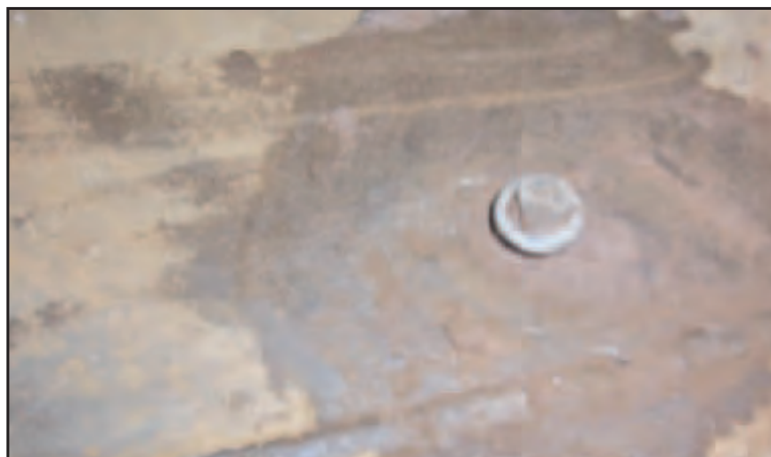
FIGURE 2. Internal corrosion so severe the tank could not be repaired for lining. The assessment of this tank predicted uniform corrosion.
