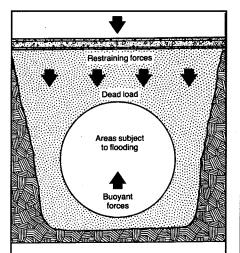
Areas subject to flooding. Tanks are typically buried three to four feet below finished grade to provide adequate slope for piping and protection from traffic loads. Except in areas with high water tables, or areas subject to flooding, the weight of backfill and pavement over the tank is sufficient to offset buoyance and prevent flotation.
