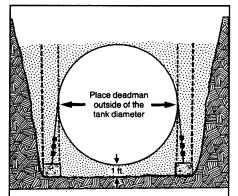
**Deadmen Anchors.** Deadmen anchors increase the amount of backfill bearing down on the tank to offset buoyancy. Deadmen anchors are convenient to use and reduce the work required to be done in the excavation.
