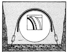
Botton hold-down pad. A reinforced bottom hold-down pad provides a firm bed for the tank and adds resistance to flotation. Insulating material separates straps from the tank. TANKS SHOULD NEVER BE SET DIRECTLY ON A BOTTOM HOLD-DOWN PAD.
