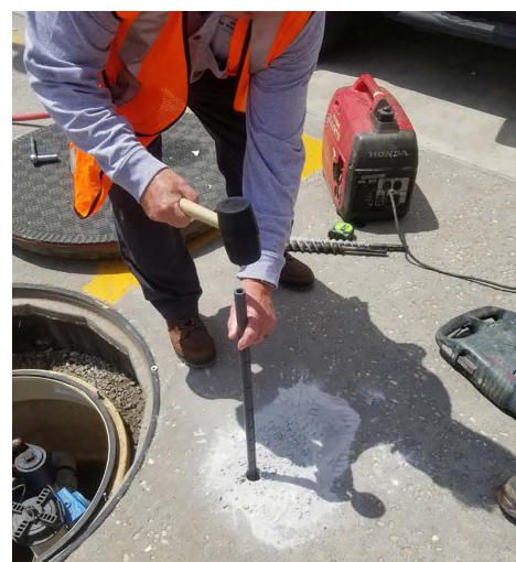
Figure 1. In the Dri-Sump method of sump testing, Vapor Stimulating Tubes (VSTs) are first driven into holes drilled in close proximity to the sump(s) to be tested. During the test, a vacuum is applied to these tubes. If any holes are present in the sump, the aerosol is drawn through the hole, into the backfill, into the VST, and then into a box where a laser beam reveals the presence of the aerosol.
