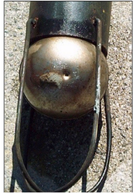
Figure 1. Removing overfill devices may reveal damage that is not otherwise obvious. Close inspection is required to detect ball floats that are stuck in their cages (left photo) or punctured so that they don’t float (right photo). Photos courtesy of Spruce Wheelock.
