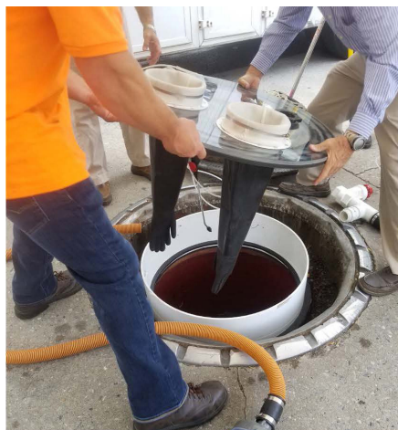
Figure 4. In the Leak Detection Technologies method of sump testing, a temporary lid with attached arms-length gloves is installed over an STP sump. The gloves allow a technician to work inside the sump while a vacuum is maintained in the sump.
