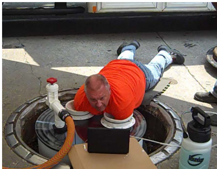
Figure 5. During the Leak Detection Technologies test, a vacuum is maintained in the sump while a technician sprays a soap solution on the sump wall and sump fittings with one hand and maneuvers a video camera in the other hand. The video image is transmitted to a screen that the technician (that's Ed in this photo) watches closely to see if any bubbles appear.
