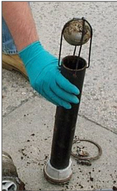
Figure 1. Removing overfill devices may reveal damage that is not otherwise obvious. Close inspection is required to detect ball floats that are stuck in their cages (left photo) or punctured so that they don’t float (right photo). Photos courtesy of Spruce Wheelock.
