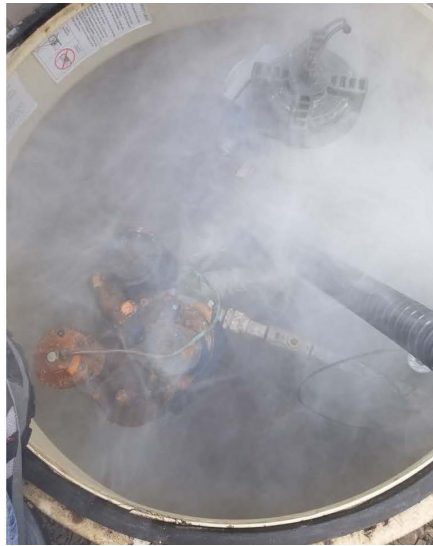
Figure 2. In the Dri-Sump method of sump testing, the sump is filled with a cloud of dense aerosol.
